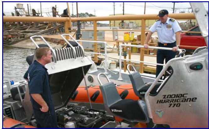
Machinery Technician 2nd Class Lance Hufford (left) shares a light moment with LT John Driscoll, Commanding Officer of the CGC Matagorda. The cutter’s conversion included installation of a stern ramp for the launch and recovery of a new seven-meter, 315-hp Short Range Prosecutor small boat, shown here. United States Coast Guard/Gordon I. Peterson
